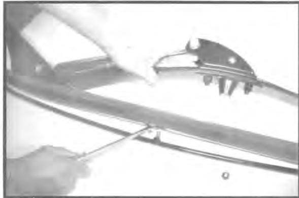
NOTE: EACH TIME A MACHINE COMES IN FOR REPAIR OR TUNE-UP, CHECK THE SKI SKAGS FOR WEAR. TO PREVENT DAMAGE TO THE SKIS AND FOR GREATER STEERING CONTROL, REPLACE ALL SKAGS THAT ARE HALF WORN OR GREATER WITH NEW SKAGS. CHECK ALL SKI SADDLE BOLTS. IF THEY ARE LOOSE OR WORN, REPLACE WITH NEW BOLTS AND NUTS.
