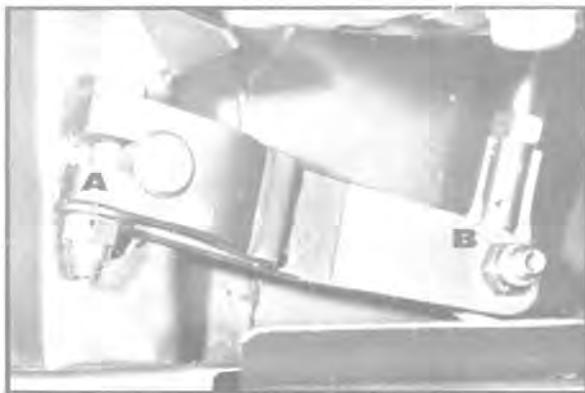
Spindle can now be removed from the body. The spindle should be lubricated annually to insure proper steering.
