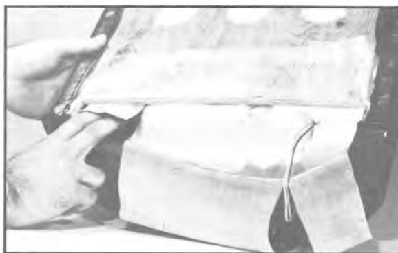
5. Place the door frame into position and install the two screws located at the bottom of door frame. Cut the material in middle of door frame as shown (A). Push the door frame securely into position (corners first). Re-rivet to compartment housing and remove excess material from compartment area. NOTE: If rivet holes were damaged when old rivets were removed, new holes can be drilled between existing holes.
